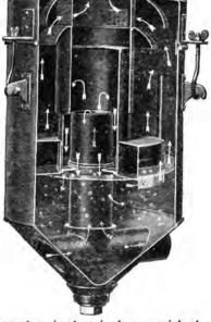
manufacture. It thoroughly cleanses the air that is drawn with the fuel into the cylinders. The air is drawn through water and two screens, the latter preventing bubbles from carrying dust through the carburetor to the motor. In this way all grit is removed and a clean, moist, highly explosive mixture is delivered to the cylinders.
